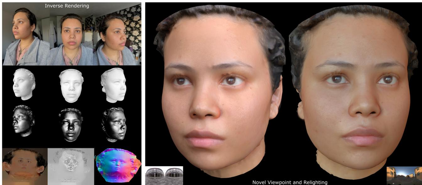
**Figure 1:** From casual smartphone frames (left, top) in arbitrary unknown lighting, our inverse optimization uses tiny shading networks to efficiently factorize light transport (left, middle) and disentangle shading from explicit reflectance maps (left, bottom). The resulting asset (mesh & textures) can be used in common pathtracers to render novel viewpoints and lighting (right).
