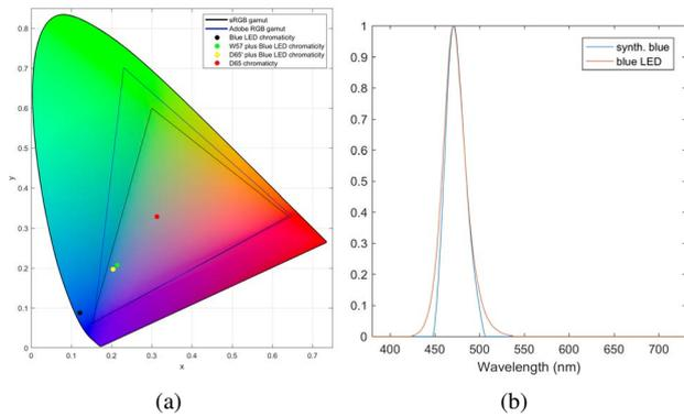
**Figure 6:** (a) The chromaticity of the narrow band blue LED lies outside both the sRGB ITU-R BT.709 and Adobe RGB colour spaces. Mixing the narrow band blue LED with a broadband illumination (D65' or W57) reports the chromaticity of the illumination within both gamuts. (b) Additional advantage is that the spectrum of the synthesized blue is narrower than the actual blue LED, contributing to sharp details correlated with melanin concentration.
