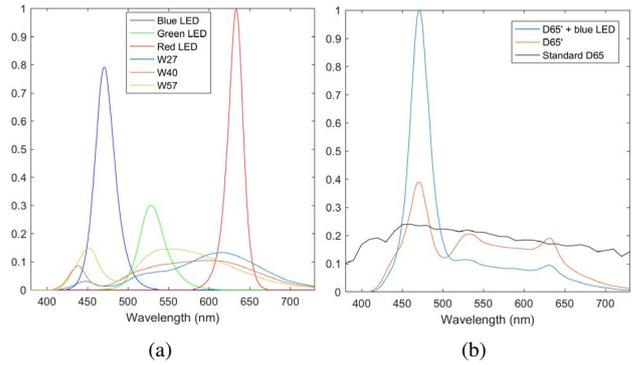
**Figure 4:** (a) Spectral power distributions of the 6 different LEDs installed on the multispectral LED sphere. (b) Spectra of D65' and D65' + blue illumination, jointly used to isolate the blue response (Section 4.2).
