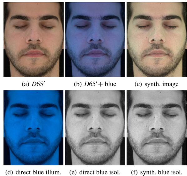
**Figure 5:** Proposed practical spectral measurements of skin reflectance (a, b). (a) Broadband D65 metamer (D65') illumination. (b) Mix of D65' + blue LED illumination. (c) Synthesized response to pure blue LED illumination, and its isolated blue channel data (f) employed for parameter estimation. (d) Direct measurement of skin response to blue illumination, and its isolated blue channel data (e).
