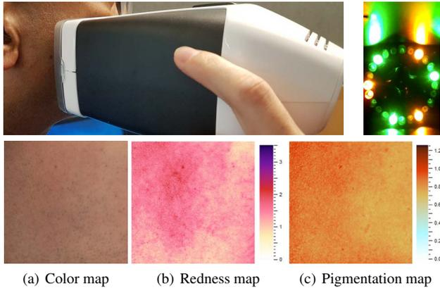
**Figure 9:** Measurement of a subject's cheek with the Antera 3D<sup>®</sup> (top) and example of acquired chromophore maps (bottom). Photograph of the device's multi-LED illumination setup surrounding the camera lens (top-right).
