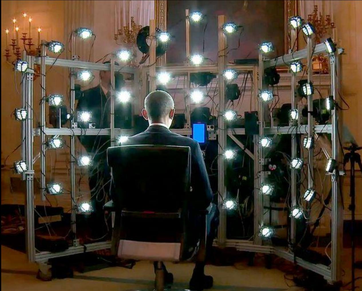
President Barak Obama scanned with portable light-stage for multi-view capture with polarized spherical gradient illumination
