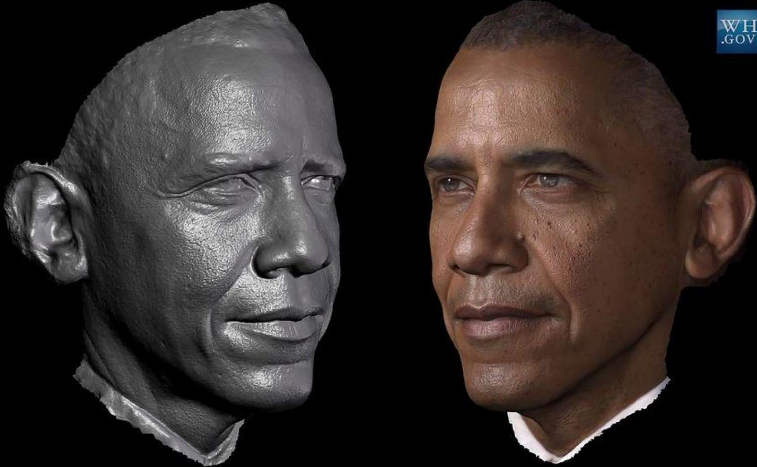
President Barack Obama scanned with portable light-stage for multi-view capture with polarized spherical gradient illumination
