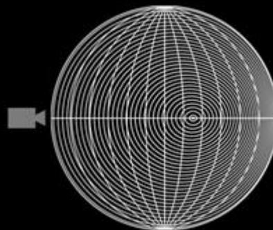
Linear polarization pattern [Ma et al. 07]
