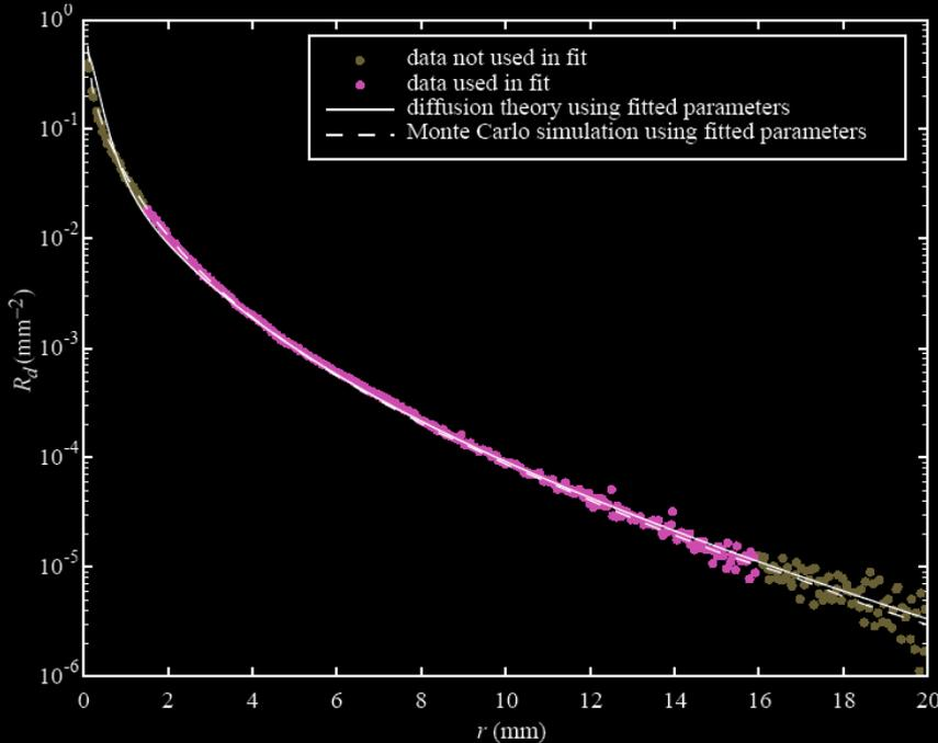
$$R_d(r) = \frac{\alpha'}{4\pi} \left\{ z_r \left( \sigma_{tr} + \frac{1}{d_r} \right) \frac{e^{-\sigma_{tr} d_r}}{d_r^2} + z_v \left( \sigma_{tr} + \frac{1}{d_v} \right) \frac{e^{-\sigma_{tr} d_v}}{d_v^2} \right\}$$
