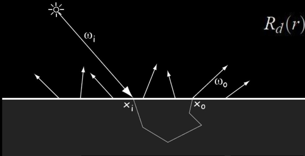
$$R_d(r) = \frac{\alpha'}{4\pi} \left\{ z_r \left( \sigma_{tr} + \frac{1}{d_r} \right) \frac{e^{-\sigma_{tr}d_r}}{d_r^2} + z_v \left( \sigma_{tr} + \frac{1}{d_v} \right) \frac{e^{-\sigma_{tr}d_v}}{d_v^2} \right\}$$
