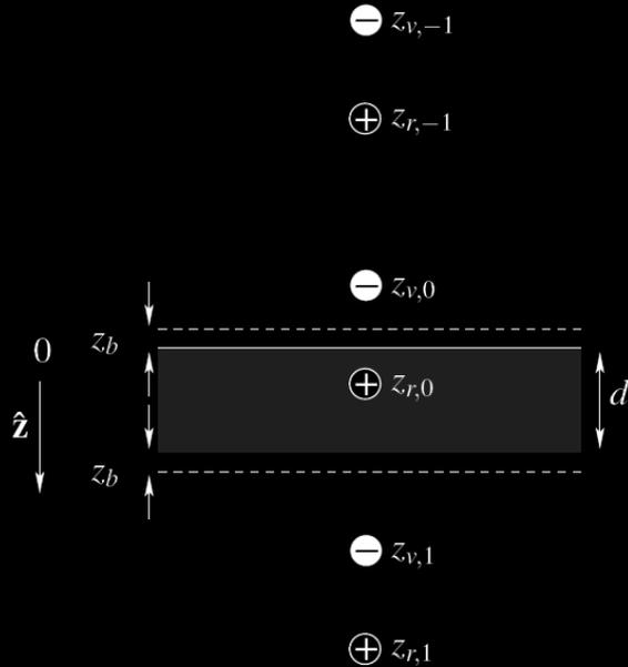
$$R(r) = \sum_{i=-n}^n \frac{\alpha'_{z_{r,i}}(1 + \sigma_{tr}d_{r,i})e^{-\sigma_{tr}d_{r,i}}}{4\pi d_{r,i}^3} - \frac{\alpha'_{z_{v,i}}(1 + \sigma_{tr}d_{v,i})e^{-\sigma_{tr}d_{v,i}}}{4\pi d_{v,i}^3}$$
